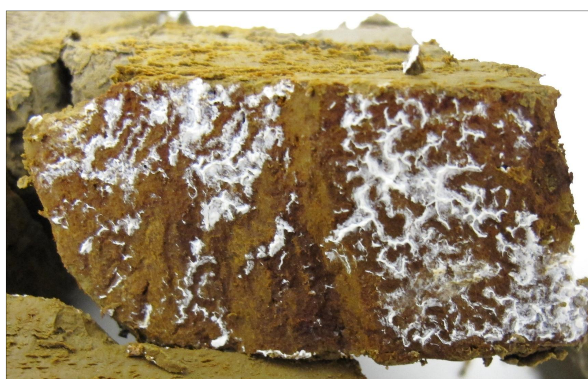
Figure 6. Suspension retained in the soil pores.
