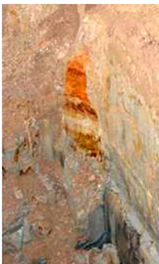
Fig. 1. Vertical profile of acid sulfate soil showing (from top to bottom) top soil, oxidized material, the oxidized/unoxidized boundary, and dark grey metal sulfides. Photograph courtesy of Rainer Rosendahl.
