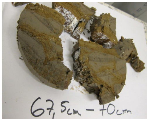
Fig. 3 (on the right). Cross-section of a soil sample after the flow of 6.4 dm 3 of calcium carbonate suspension through the column during eight days.
